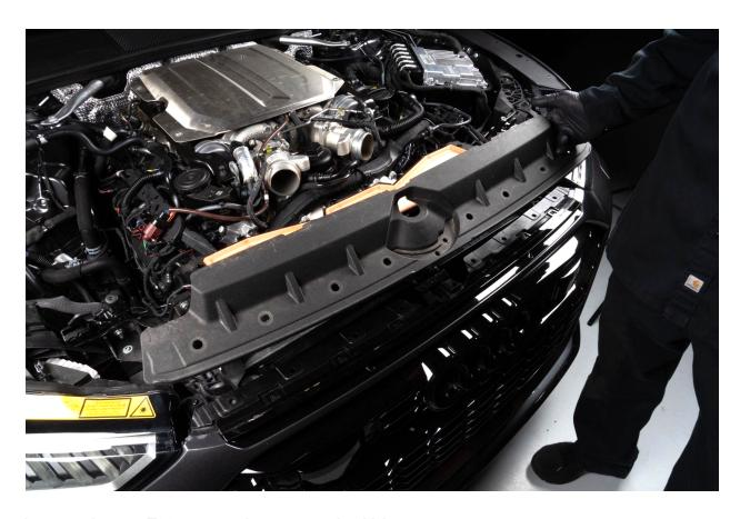
Loosen the two T30 screws that secure the Airbox
