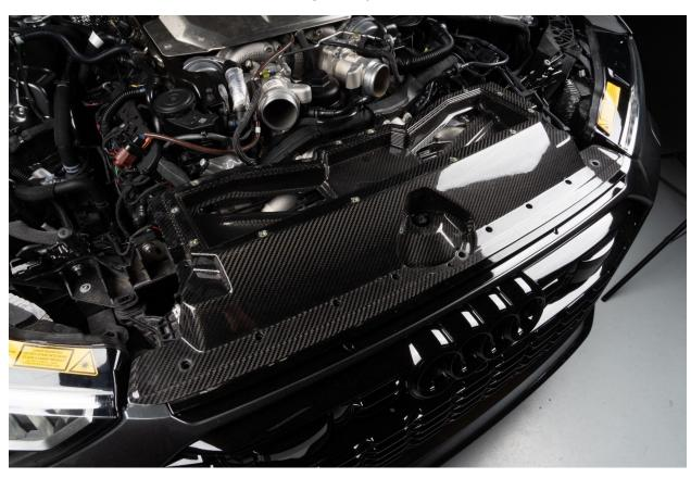
Reinstall 9 Push in retainers on the front edge of the intake
