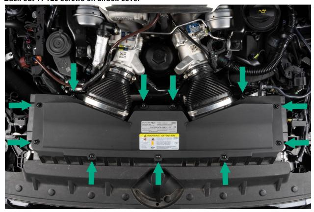
Loosen both turbo inlet clamps with flat head screwdriver, then pull off of turbo inlet.
