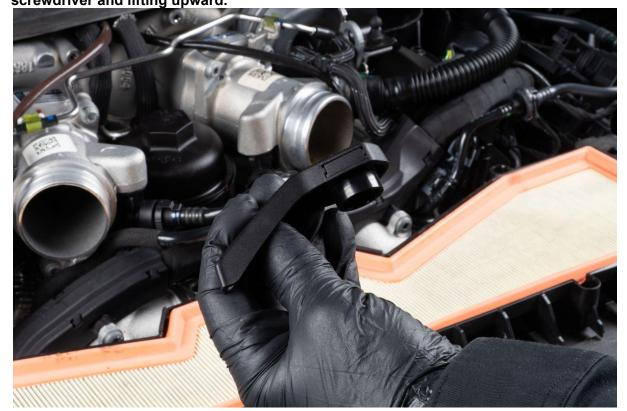
Remove 9 Push in retainers from the front trim piece. Set the retainers aside to be used later.
