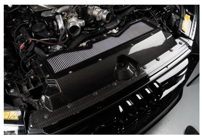
Install two 4mm button head screws and washers on the outside edge of the airbox using hand tools. Do not over-tighten. Snug is fine.
