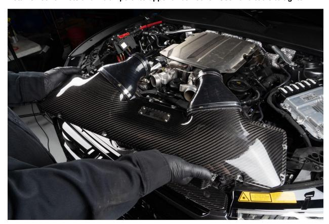
Place the upper airbox cover in place on top of the lower box while simultaneously sliding the silicon onto the turbo inlet. Leave silicone clamps loose fitting for now.
