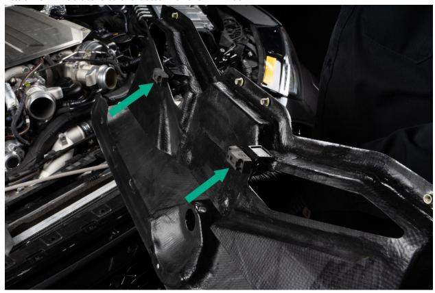
Place lower portion of airbox into the engine bay and secure with push in retainers
