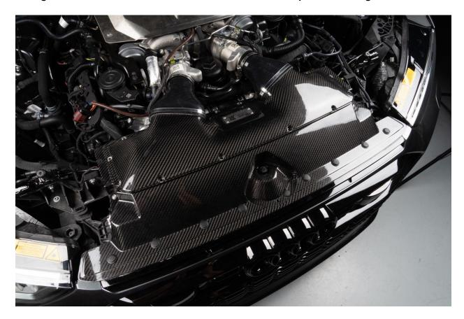
Loosely install twelve 3mm button head screws and washers to attach the upper airbox cover to the lower airbox cover. Once all screws are in place, tighten down with hand tools. Do not over tighten.
