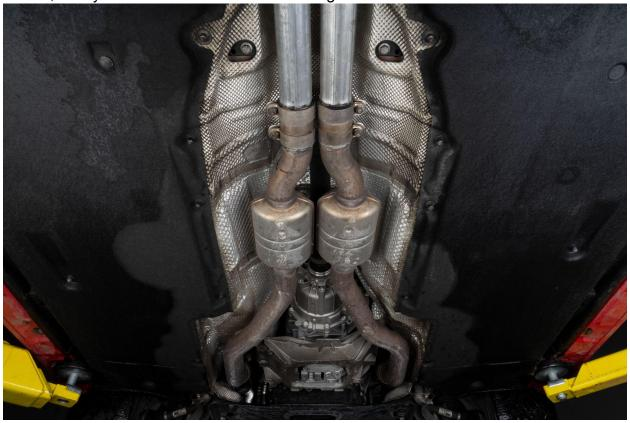
Loosen four 13mm nuts that connect the Midpipes to the rear muffler section of the exhaust.
