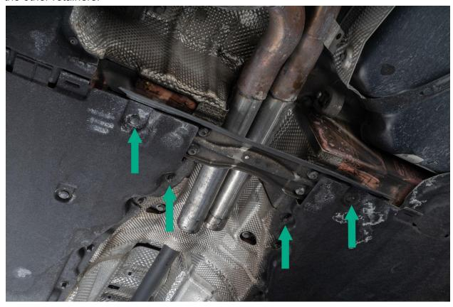
Remove eight #10 triple square bolts (4 on each side) that secure the cross support.
