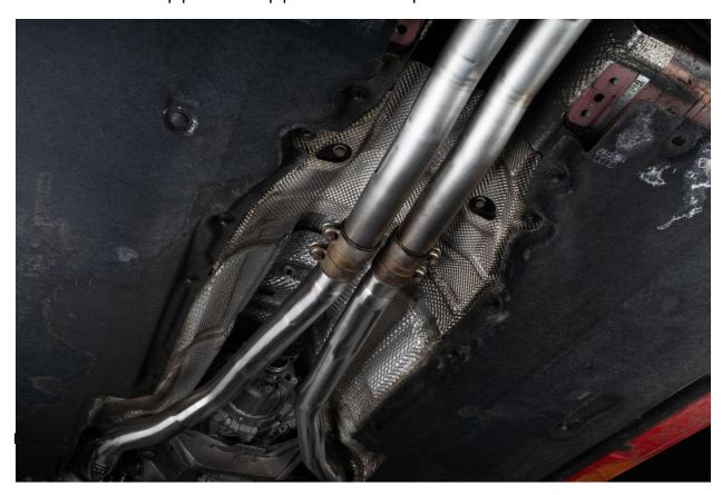
Make final adjustments then tighten all exhaust clamps.
