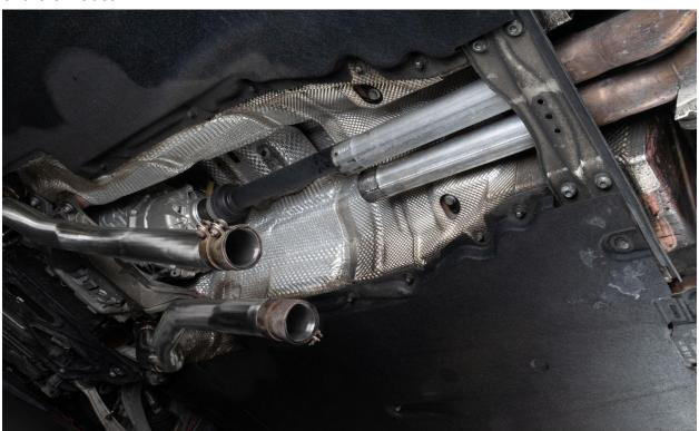
Hold the IE x-pipe up to the factory exhaust making sure to keep the front lined up and level with the front of the OEM pipe that was just disconnected from the midpipes. There is a sticker on the X-Pipe to ensure proper orientation. Once it is in place, mark where the x-pipe ends on the factory rear exhaust section. This step can only be properly done once so remember to old adage, "Measure twice, Cut once".
