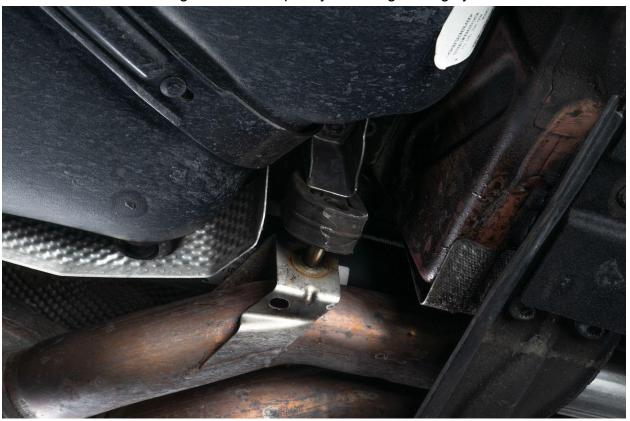
Slide provided exhaust clamps over Axel back portion of the exhaust and loosely insert IE X-Pipe.
