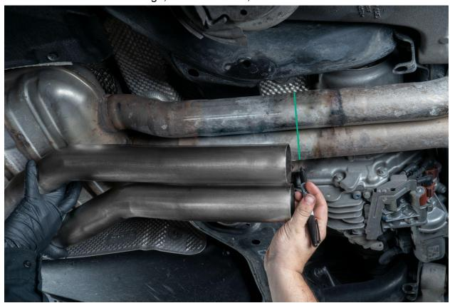
Using a saws-all, cut where you marked in the last step. (Exhaust pictured is not OEM)
