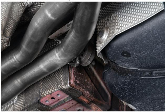
Insert the front of x-pipe into midpipe exhaust clamps.
