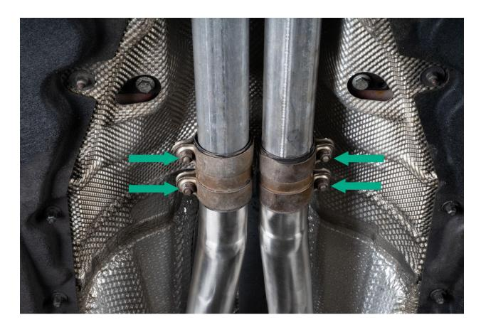
Push the exhaust clamps forward onto the Midpipes to disconnect from the rear section of the exhaust.
