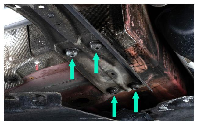
Using a large flat head, pry off the exhaust hangers on each side. **Take care**. When the exhaust is free of the hangers it will fall quickly and weighs roughly 15lbs.
